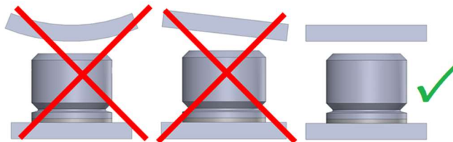
Fig. 4: counter-pressure plates even and parallel moving
